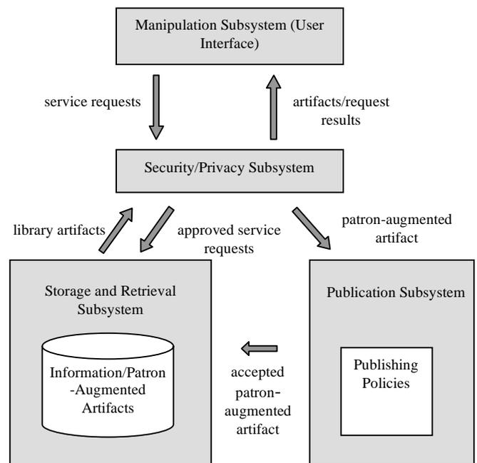
Fig. 4. Conceptual architecture of Synchrony.
